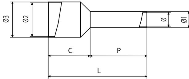
**TWIN END SLEEVE, PRE-INSULATED WITH PA6, WHITE, FOR FLEXIBLE COPPER CONDUCTORS, SECTION 2X0,5MMQ P=8MM**
